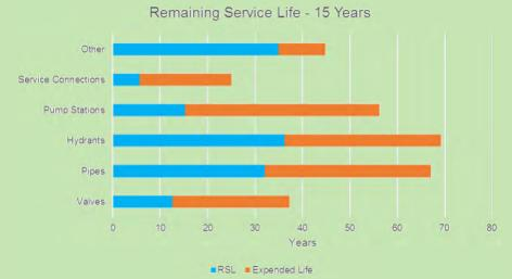
Figure 2-2: Remaining Service Life of Water System Components
