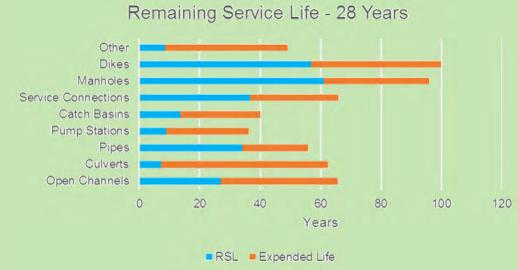
Figure 4-2: Remaining Service Life of Drainage System Components
