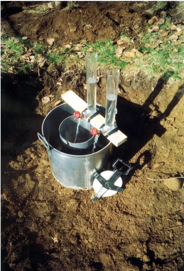
Photo 2. Double ring infiltrometer installed at Site #10.
