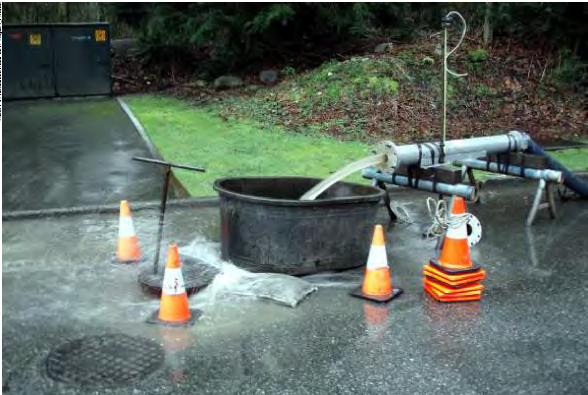
Photo 7. Well discharge configuration during aquifer pumping tests, Feb. 15, 2011.
