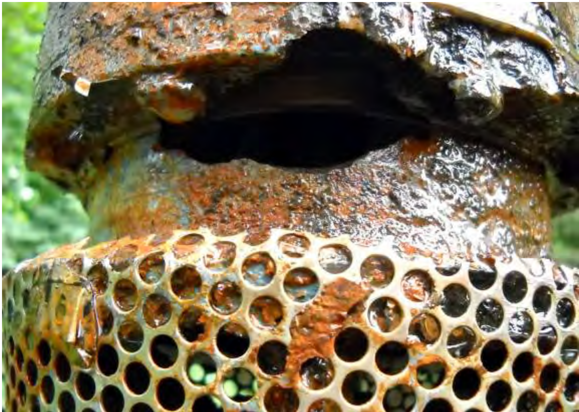
Photo 6. Damaged pump pulled from Maple Creek well in September 2010.
