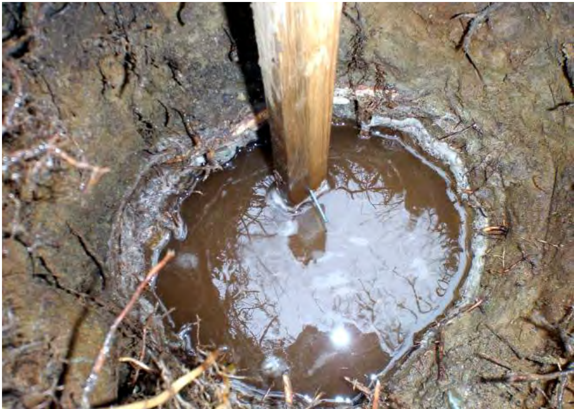
Photo 12. Percolation test at foot of Ozada Ave., near school.
