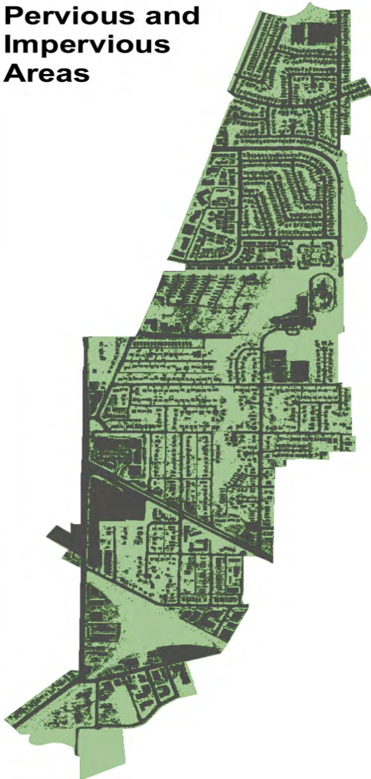
Figure 2-6: Existing Pervious and Impervious Areas from 2010 Ortho photography
