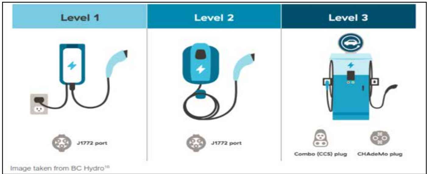
Figure 12.5: Level 1, 2 and 3 Charging Types
