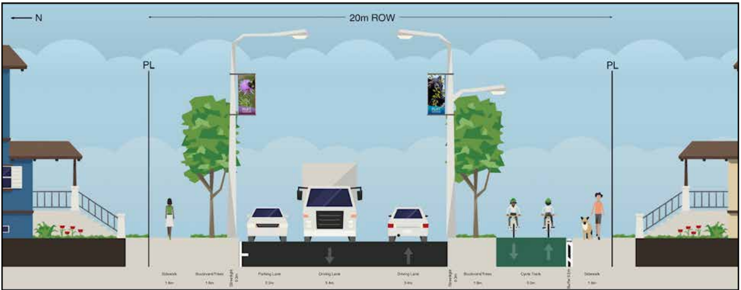
Figure 9.1b: Lincoln Avenue Corridor - Typical Cross Section
