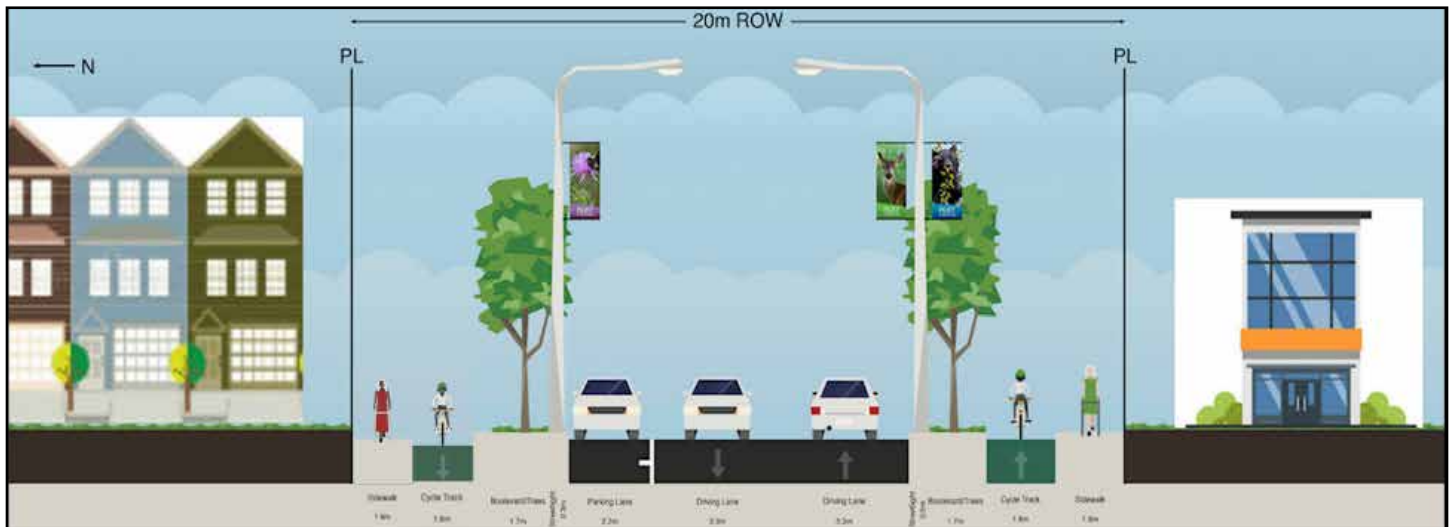
Figure 9.1d: Dominion Avenue Corridor - Typical Cross Section
